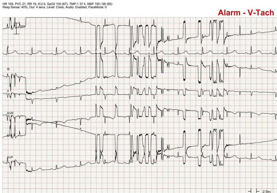
FIGURE 53.5 Electrode failure causing artifact and a false ventricular tachycardia alarm (V-Tach). Electrocardiogram in six of the seven available leads shows intermittent loss of signal (signal “squares off” on top and bottom of tracing) due to an electrode problem such as loss of skin contact or dried out electrode gel. One ECG lead (lead II that uses the right arm and left leg electrodes) does not show electrode failure so the likely electrode that is malfunctioning is the left arm electrode. Failure to apply fresh electrodes in this case will result in numerous false alarms. Drew BJ, Harris P, Zegre-Hemsey JK, Mammone T, Schindler D, Salas-Boni R et al. Insights into the problem of alarm fatigue with physiologic monitor devices: a comprehensive observational study of consecutive intensive care unit patients. PLoS One. 2014;9(10):e110274.
